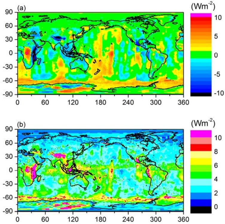
Figure 4-4. (a) Mean and (b) RMS difference between SW TOA fluxes from CERES Terra and CERES Aqua SYN1deg Ed2.6 data products.
